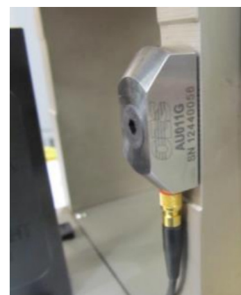
Typical Piezo Strain Sensor Mounting locations – Steel Frame and Cast Iron Frame Presses
